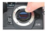
Grasp the frame of the filter with the non OM SYSTEM branded side facing up, and set it with the notched part of the frame facing downward. Gently press the frame with your fingers to evenly insert the filter, ensuring it is parallel to the sensor. Avoid applying excessive force during this process. Also, be careful not to touch the electrical contacts or sensor on the camera. OM SYSTEMの刻印のない面を表側にして、フィルターのフレーム部をつまみ、
