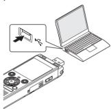
Press the ►OK button to start charging the battery.
